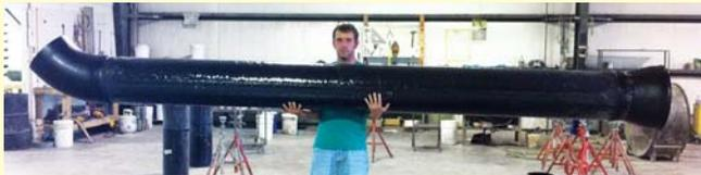
Fiberglass drain piping can be up to 10 times lighter than equivalent metallic systems. This allows the installer to reduce the crew sizes required on-site as just one laborer can handle full sticks of pipe and fittings. Even though the material is light, the mechanical properties of fiberglass still fall more closely in line with steel products rather than weaker thermoplastics like PVC.
